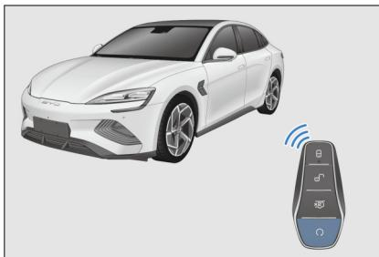
3. Press and hold the remote start/stop button on the electronic smart key for two seconds. The vehicle stops and powers off, and turn signals flash twice.
